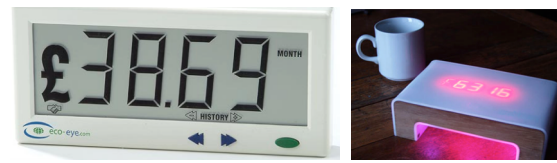
Figure 3. The Eco-Eye [10] (left) provides direct feedback on household electrical consumption, while the Wattson [7] (right) additionally provides ambient feedback. (Eco-Eye image courtesy of Modern Moulds and Tools Ltd.; Wattson image courtesy of DIY Kyoto. Used with permission.)
